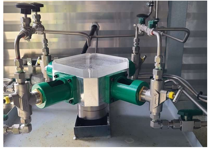
Electric chemical injection pump – zero emissions
