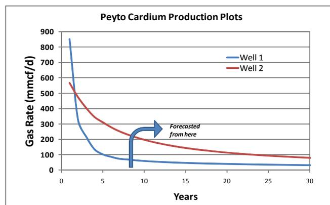
Well #1 is a faulted Cardium well (see figure 2) that has a relatively tight or low matrix permeability feeding that fault system. Even with a large fracture stimulation during the completion, to connect to the natural fractures that the fault creates, the well will ultimately deplete at the rate the matrix permeability provides (permeability being the measurement of a rock's ability to transmit fluids).
